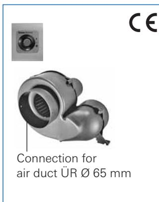
For warm air distribution of the heater Trumatic S 2200, as an additional fan for increasing the air output in particularly long warm air duct systems or as an extractor fan in the kitchen or bathroom (in conjunction with an intake nozzle DM).
