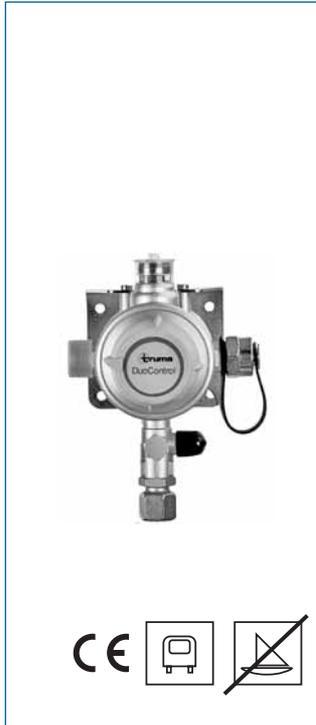
The wall-mounted **DuoControl** changeover regulator system for the two-cylinder system with integrated gas pressure regulator and test connection can only be used if **heating is not required** while driving (in vehicles as of 2007).
