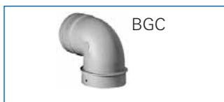
34091-01 Elbow **BGC** for direct connection to the warm air outlet (outlet for air ducts Ø 65 or 72 mm)
