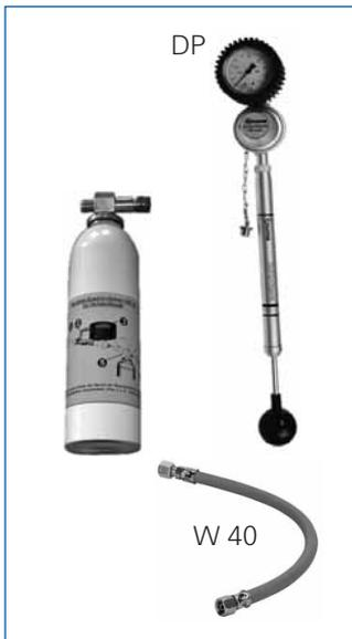
54100-00 Leak testing kit **DP**, Pressure pump with pressure gauge for leak testing liquid gas systems in vehicles or boats. c/w a protective bag and sealing nipple for testing two-cylinder gas units (pressure limitation at approx. 150 mbar)
