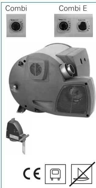
Heater (excluding exhaust duct) with thermostat, control panel with 3 m connecting cable, mounting parts, currentless FrostControl safety/drain valve and elbow fittings for 10 mm diameter water hoses. Models with water connections for semi-rigid piping (John Guest System) on request.
