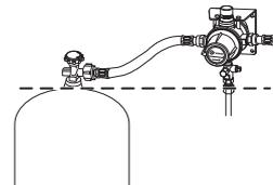
DuoControl should be installed so that the high-pressure hose connections are in the highest possible position, and at least above the cylinder valve level (broken line).
