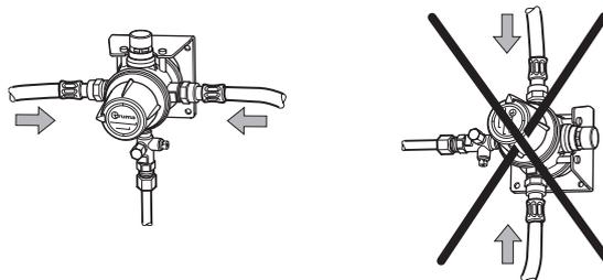
The DuoControl changeover regulator must always be installed in such a way that the high-pressure hose connections are arranged in a **horizontal** position.
