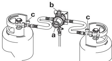
The mica window (b) indicates the status of the operating cylinder:
