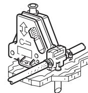
**!** To allow safe drainage of the content of the boiler if there is a risk of frost, an automatic aeration valve must be fitted to the warm water supply of the boiler. Standard for all warm water devices from Truma.
