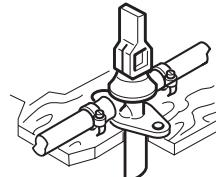
For the Trumatic C heating system, the FrostControl replaces the electrically operated safety/drain valve ELASI.
